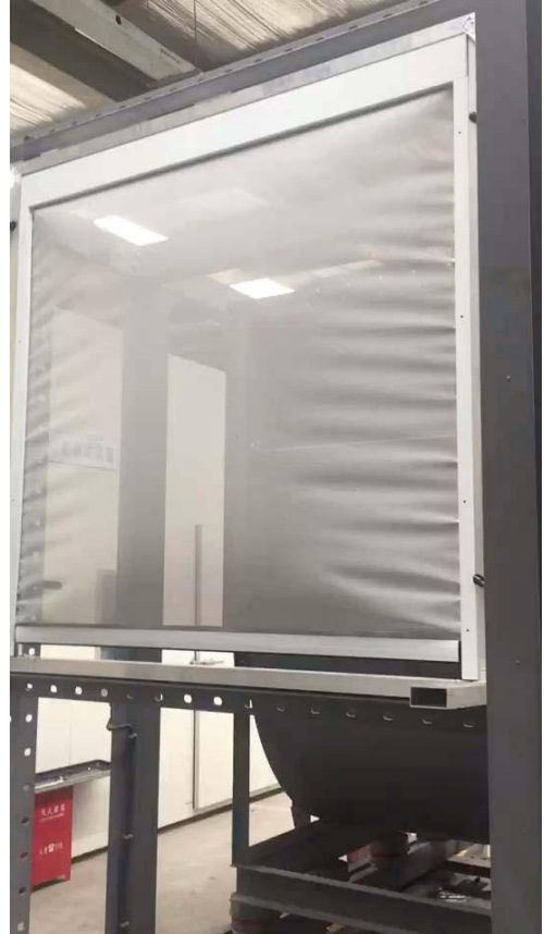
Dynamic wind pressure test level 12 wind (35m / s)
